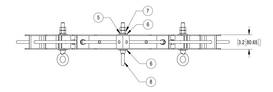
NOTE: 1 - MAXIMUM NET CABLE WEIGHT FOR STRAIGHT POLES: A- PER EYEBOLT = 1000 LBS B- PER MOUNT = 3000 LBS 2 - MAXIMUM NET CABLE WEIGHT FOR TAPERED POLES: A- PER EYEBOLT = 1250 LBS B- PER MOUNT = 3750 LBS 3 - REVIEWED FOR USE WITH A MINIMUM POLE DIAMETER OF 10" WITH WALL THICKNESS OF 3/16" AND A YIELD STRENGTH OF 36 KSI. FOR USE ON THINNER MATERIAL REQUIRES ADDITIONAL ENGINEERING REVIEW
