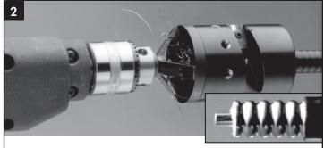
Position the tool on the cable so that it is aligned and start the drill at medium to full speed. Use slight and steady pressure to force the tool along the cable until you feel the detent action as the ball bearings snap into place. The pitch of the motor will also increase. Then, stop the motor, switch to reverse, and withdraw the tool. **Note:** Reversing the motor prevents the cutter blades from striking the outer conductor should the motor accidentaly be restarted.
