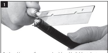
Cut the cable square. If necessary, bend the cable slightly at about 5" (127 mm) for more gripping leverage. **Note:** Do not exceed the minimum bend radius of the cable.
