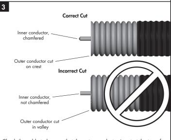
Check the cable to be sure that the outer conductor is cut at the top of a crest, that all cuts are clean, that the inner conductor is chamfered, and there is no debris on the surfaces.
