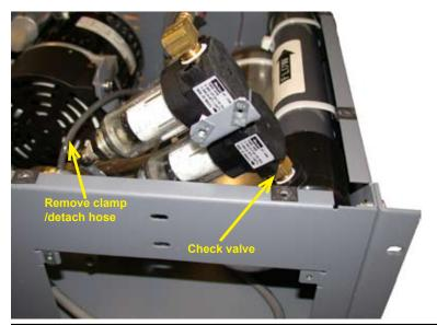
Step 4 Remove clamp from hose and detach hose from barb fitting on the bottom of filter assembly.
