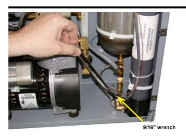
Step 3 Loosen compression fitting (using 9/16" wrench) and detach hose from connection where shown.
