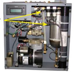
Step 2 Remove clamp from hose and detach hose from barb fitting on the filter assembly.
