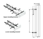
Adjustable Tilt Pipe Mounting Kit for 2.362"-4.5" (60-115mm) OD round members for panel antennas. Includes 2 clamp sets.
