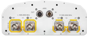
4-port sector antenna, 4x 1695–2690 MHz, 65° HPBW, 1x RET and internal Bias-T on first highband port. The two highband arrays utilize a common tilt.
