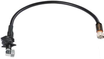
D-CLASS HELIAX® 1/2" SureFlex® Jumper with interface types 7-16 DIN Female and 7-16 DIN Male Right Angle with HELIAX® SureGuard weatherproofing, 1.5 m (boot on DR end only, and DF end no boot)
