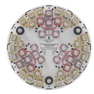
42-port Tri-sector antenna, 6x 698-896MHz, 24x 1695-2690MHz and 12x 3300- 4000MHz, 65° Horizontal Beamwidth, fixed tilt.
