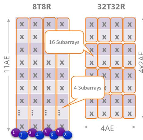
Figure 36: 8T8R and 32T32R mapping
