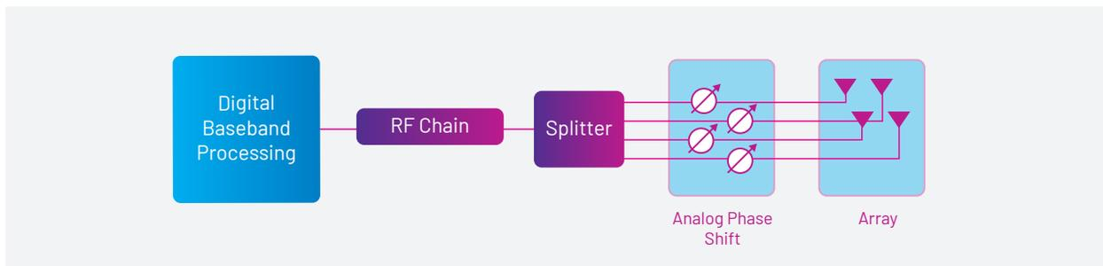
Figure 16: Analog beamforming
