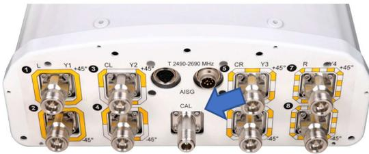
Figure 27: Calibration port on an Andrew antenna
