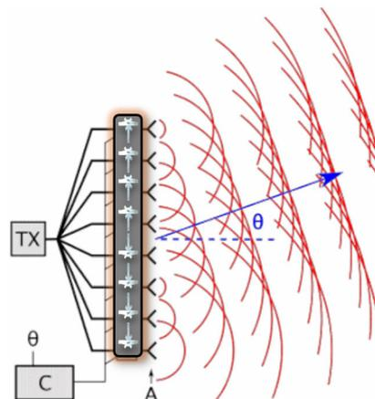
Figure 14: Effect of phase shift
