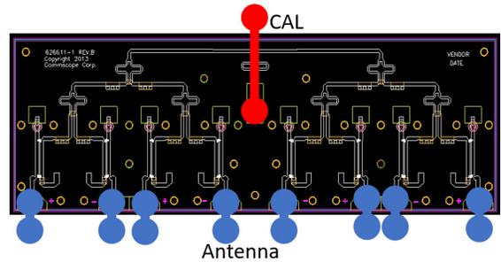
Figure 28: Calibration board
