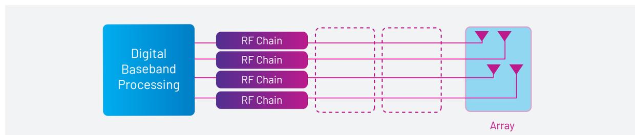
Figure 17: Digital beamforming
