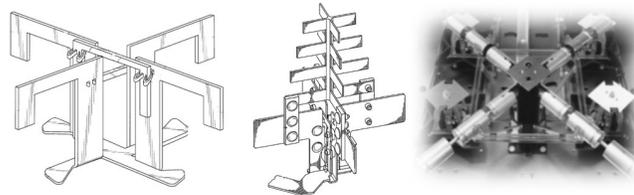
Figure 9: Andrew patented antenna element examples
