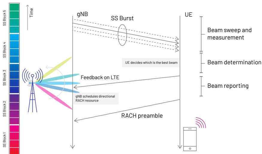
Figure 2: Initial access in NSA mode [3]
