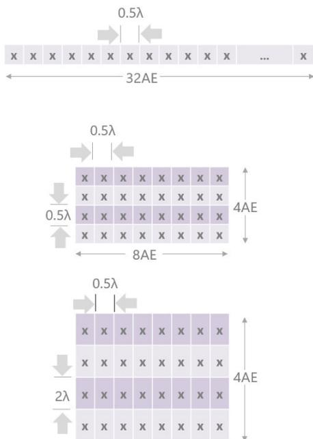
Figure 37: 64T64R mMIMO panel configuration
