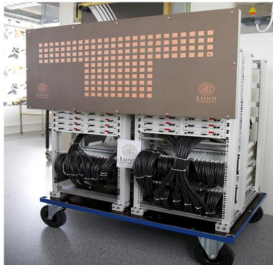
Figure 32: The Lund University massive MIMO testbed—(LuMaMi)
