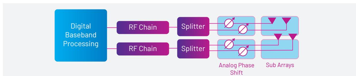
Figure 18: Hybrid beamforming
